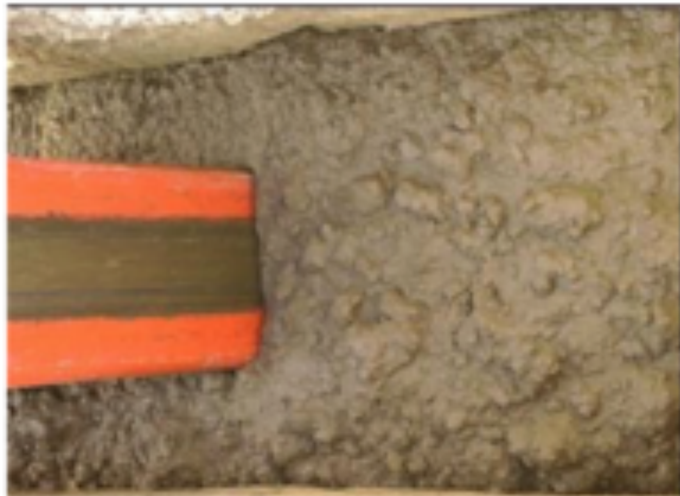
Geomix Excess material < 30% of treated volume
