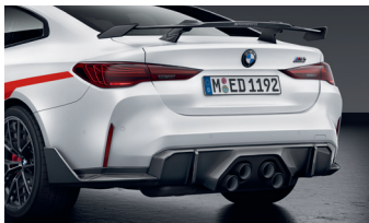
Carbon Rear Winglets, Carbon Rear Diffuser With M Performance Silencer System And Titanium Tailpipe Trims Module
