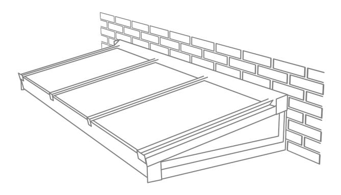
Drawing 1: Make a recess in the roof where B = the ordered width and L = the ordered length of the skylight. It is recommended to provide the skylight with lead finishing on the wall. For this, make a recess where [M=L+340 mm] and [H=the total height of the skylight+50 to 100 mm].
