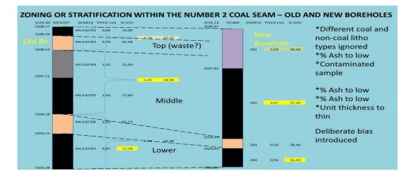
Figure 3: Illustration of the inconsistent sampling methodology employed in borehole Area 1-09
