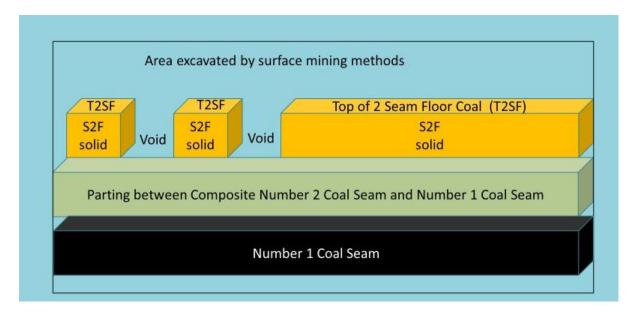
Figure 14: Illustration of uneven pit floor after Beta Coal Seam Select has been removed
