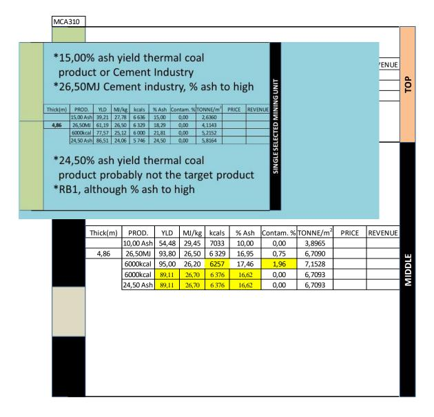
Figure 7: Illustration of different products from stratified Beta Coal Seam Borehole Z
