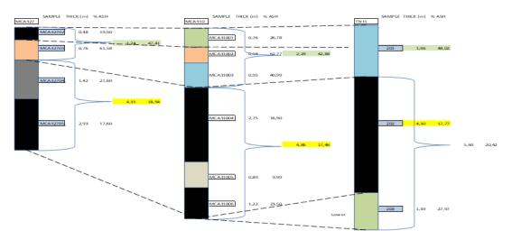
Figure 1: Illustration of the stratification profiles within the Beta Coal Seam. Please take note that the figure is not a geological cross-section.
