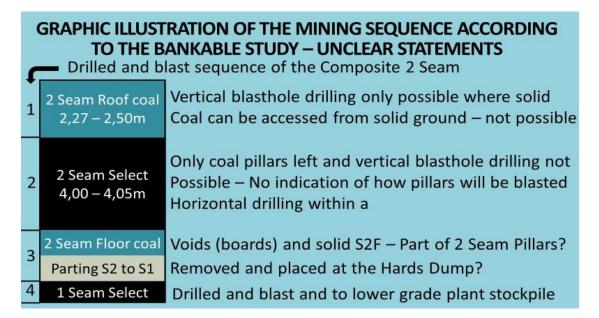
Figure 12: Illustration of the planned mining sequence of the Composite Beta Coal Seam
