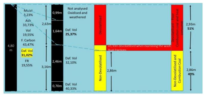
Figure 10: Illustration of methodology to investigate devolatilisation characteristics present in a coal deposit
