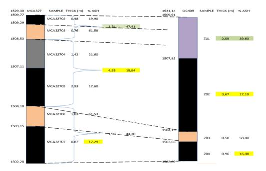
Figure 2: Illustration of the inconsistent sampling methodology employed in borehole Area 1-01 with TN11 as the old control borehole
