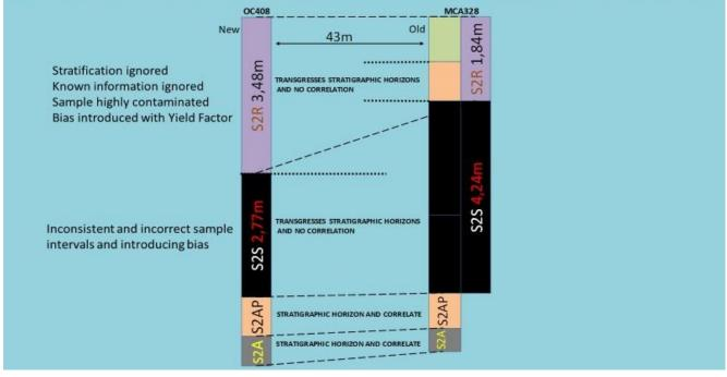
Figure 4: Illustration of the conflicting sampling methodology employed in Borehole Area 1-08
