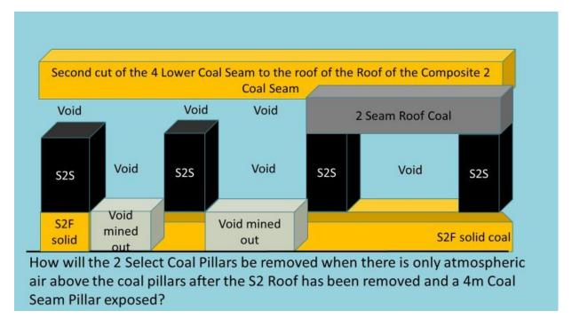
Figure 13: Illustration of voids and partial and solid coal pillars in relatively complex mining environment
