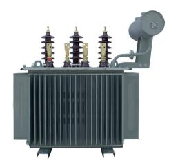
Transformers with Oil Type Expansion Tank are manufactured with powers between 25-5000 kVA up to 36 kV system voltage. Standard type 3-phase oil naturally cooled (ONAN) transformers can be used internally (Plug-in type insulator) and external (Porcelain type isolator). According to the special requests of the customers, special productions are also made for the no-load running tap changer and other cooling systems. (ONAF-ODAF etc.)
