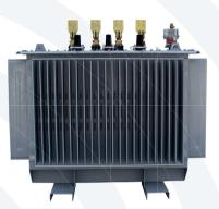
Oil Type Hermetic Transformers are manufactured with powers between 25-5000 kVA up to 36 kV maximum system voltage. Standard type 3-phase oil naturally cooled (ONAN) transformers can be used internally (plug-in type insulator) and external (porcelain type isolator). Special productions are also made for the no-load running tap changer and other cooling systems according to the special requests of the customers. (ONAF-ODAF etc.)
