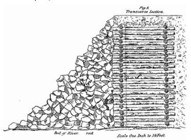
Left: a profile view of a typical Timber Crib Dam showing large stones piled on the upstream side. Illustration from "Rideau Dams", by Lieutenant W. Denison, in "Papers on Subjects Connected with the Duties of the Corps of Royal Engineers", London, 1838.
