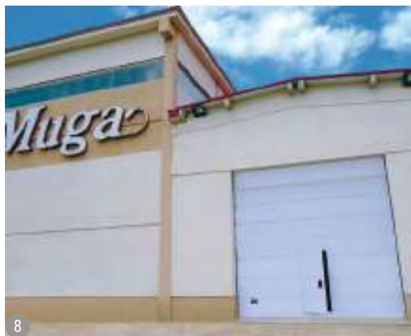
8/ SECTIONAL DOOR WITH WICKET GATE.
