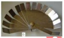
The measurement method differs from that of a "gauge ball" in that the distance between the undersides of the nail's tip is measured, and like the "gauge ball", the distance between the undersides of the nail is determined by the feeling of whether it is touching or not. Like in image C. "Plate gauge" sizes are in 0.25mm intervals (other sizes are also available).
