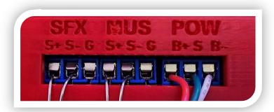
The speakers should be 4 Ohm 5 Watt or better and can be wired as mono or stereo. A single speaker may be connected to the SFX or MUS connections by using S+ and S-, if you want to use 2 speakers per channel you can connect speaker 1 positive to S+ and speaker 2 Positive to S- and both speakers' grounds to G (Ground). And you can do this for both SFX and MUS or you can mix and match if you want to use 3 Speakers. Each sound channel is separate.
