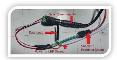
This shows one way to do the power injection using a off the shelf power supply from amazon.
