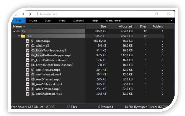
The files on the SFX MicroSD card are numbered and required to be numbers like this for the system to find the correct file for the correct function.
