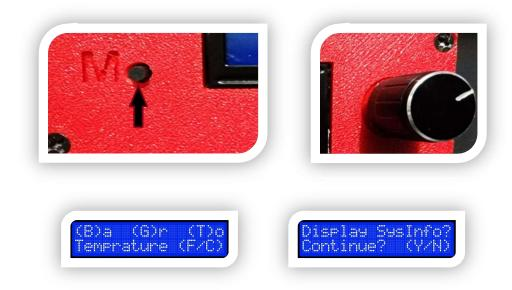
To select an item on the display, use the rotary knob. Once you've highlighted the desired item, press the rotary knob inward to confirm your selection. You can also skip the delay between screens by pressing the knob when an information screen is displayed, as shown below.
