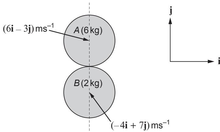
Immediately after the collision, sphere *B* has velocity  $(-4\mathbf{i} - 5\mathbf{j}) \text{ ms}^{-1}$ .
