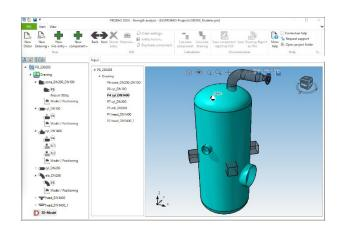
Important parameters of the components like materials, dimensions referring to standards as well as load cases are taken over into the calculation modules.
