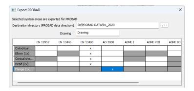
The entire project structure is generated by the specified calculation modules. The structure is subdivided in accordance with the particular standard.
