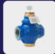
2TGA.B, 2TGA.BT DN: 20-50 Temp: -5°C to 120°C Kvs: 5-30
