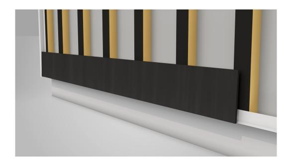
After installing the start/ventilation profile, the Fiberplank start panel must be screwed on. This plank is 1800x180x8 mm. The starting panel is the same color as the Fiberplank siding. After installing this starter board, the construction parts will not be visible through the cutouts in the Fiberplank boards. When joining panels, a gap of 1-2 mm is necessary.
