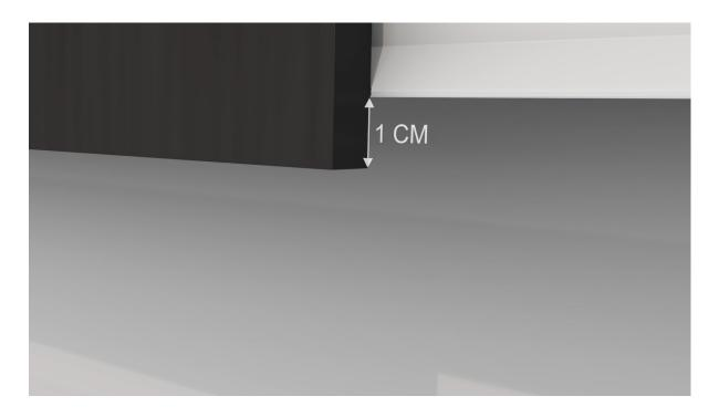
The starting panel must be lowered 1 cm below the starting/ventilation profile. due to rain drainage, so that moisture does not collect on the plank and profile.
