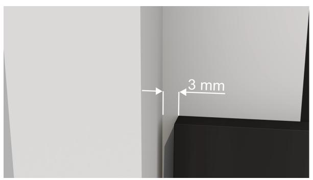
When installing Fiberplank facade boards, it is necessary to leave a gap of 2-3 mm between the boards and the finishing facade profiles that are installed in the outer and inner corners of the house.
