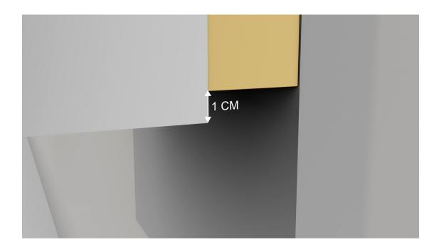
When installing the finishing profiles, place them 1 cm lower or above on the frame structure. Profiles can be cut with a metal saw or cut with metal scissors. Fasten the profiles to the frame structure with screws. Use a mechanical tools to attach the profiles straight. The ends of the profiles can be sharp, so use gloves.
