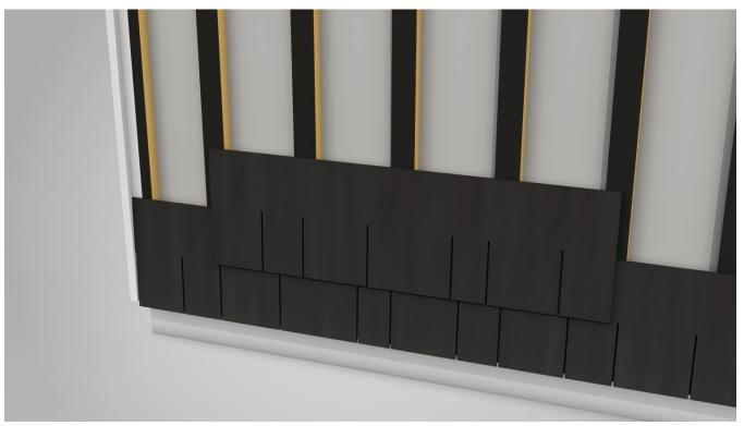
When screwing the panel, it is necessary to keep the specified distance from the edge of the panel, otherwise the edges of the panel may split. When joining panels, a gap of 1-2 mm is necessary.
