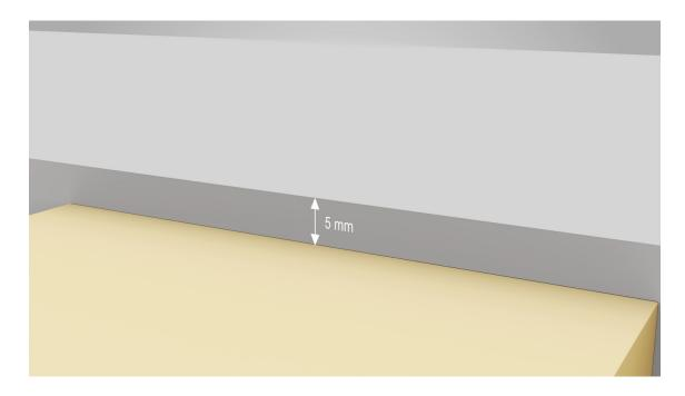
An air gap of 5-10 mm is left at the top of the frame to ensure proper ventilation of the facade. A ventilation profile is used at the top.
