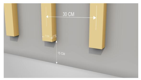
The frame is installed every 30 cm between the centers of the slats. The frame structure must be raised from the ground by 15 cm. As a standard, the slats must be at least 7 cm wide for the correct connection of the Fiberplank panels. Make sure the fasteners will support the weight of the supporting structure and Fiberplank siding.
