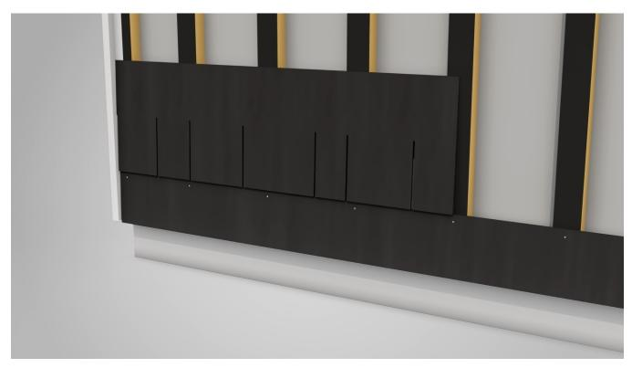
After installing the start Fiberplank boards around the perimeter of the house, it is necessary to start installing the Fiberplank facade finish with cutouts.
