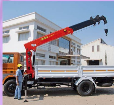
Truck Mounted Crane
