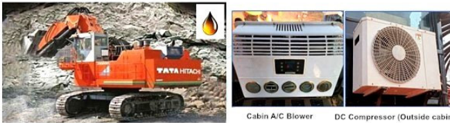
Cabin A/C Blower DC Compressor (Outside cabin)
