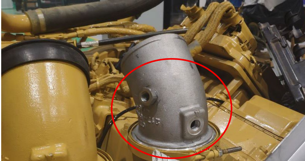
Modified Air intake duct for installation of pressure and temperature sensors
