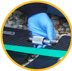
Titanium interlocking and screwing mechanism.
