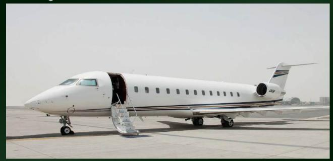
The Challenger 850 is a super-midsize private jet, seating up to 15 passengers, with a maximum range of around 2,800 nautical miles and a cruise speed of 528 mph. It has a cabin length of 48 ft 5 in, a height of 6 ft 1 in, and a width of 8 ft 2 in.
