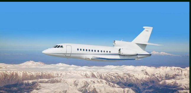
The Dassault Falcon 900EX is a long-range, tri-engine private jet known for its comfortable cabin and extensive range. It typically seats 10-15 passengers and can accommodate up to 19 with some configurations. The Falcon 900EX has a maximum range of 5,180 miles (4,500 nautical miles) and a service ceiling of 51,000 feet.
