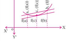
The Mean value Theorem states that there is a point c in (a, b) such that the slope of the tangent at (c, f(c)) is same as the slope of the secant between (a, f(a)) and (b, f(b)) or there is a point c in (a, b) such that the tangent at (c, f(c) is parallel to the secant between (a, f(a)) & (b, f(b)).
