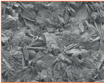
Fig. 7b: SBTC® coating after screw test in swine bone
