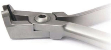
ES 475 - Distal and cutter TC with safety hold. Max 0,022" x 0,028" (0,56 mm x 0,71 mm).
