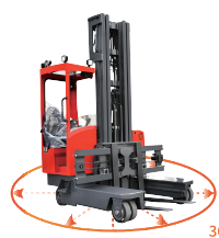
MQC25 Multi-directional Forklift ( Double drive four point, 48V ) Rated Load:2500kg Lift Height:3000-8000mm
