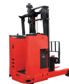
MF15/MF20 Reach Truck Rated Load:1500kg/2000kg Lift Height:3000-7500mm
