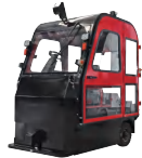
MGA60 Tow Tractor Rated Traction Capacity:6000kg
