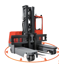
MQC35 Multi-directional Forklift ( Double drive four point, 48V ) Rated Load:3500kg Lift Height:3000-8000mm
