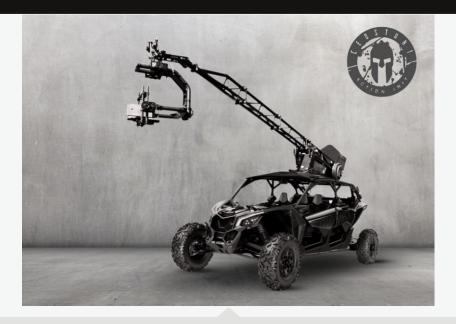
ULTRA is built for **off-road and on-road performance in the heat, snow & rain. Constructed of 6061–T6 aluminium alloy, ULTRA has the highest strength-to-weight** ratio of any compact arm. The 3 Axis isolator keeps **stabilized heads undisturbed during** aggressive use on the track.
