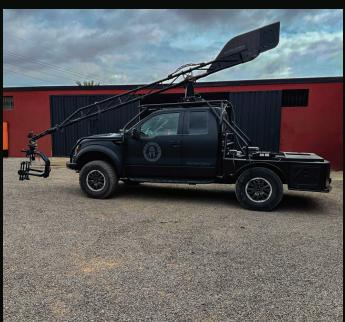
Renowned for its impressive towing capacity, the Raptor can easily A-frame other picture cars, as well as trucks and even armored military vehicles. Its versatile rear, and front platforms provide a stable base for operating any type of crane (up to a 35 foot crane) with maximum safety, making it the ideal choice for dynamic and challenging film environments.
