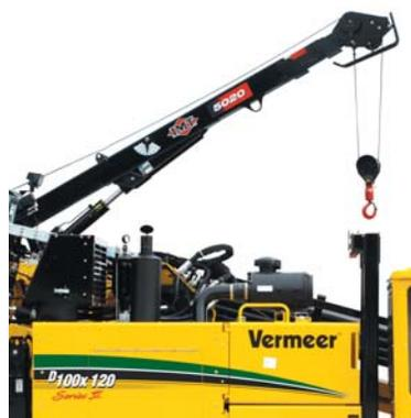
**An optional telescopic crane** allows the drill operator to change out rod boxes without the use of an excavator or backhoe. The remote-controlled crane gives the operator freedom to move around the drill for improved visibility when replacing rod boxes. The crane has a lift capacity of 7530 lb (3415.6 kg) and a maximum reach of over 20.6' (6.3 m).
