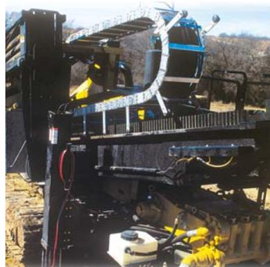
**Rack-and-pinion drive.** This simple system provides smooth operation. The D100x120 Series II unique narrow rack-and-pinion design helps maintain a small footprint for accessibility in congested areas.
