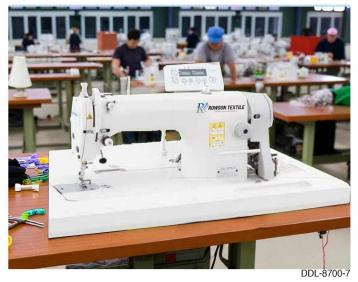
1-needle, Lockstitch Machine with Double-capacity Hook
