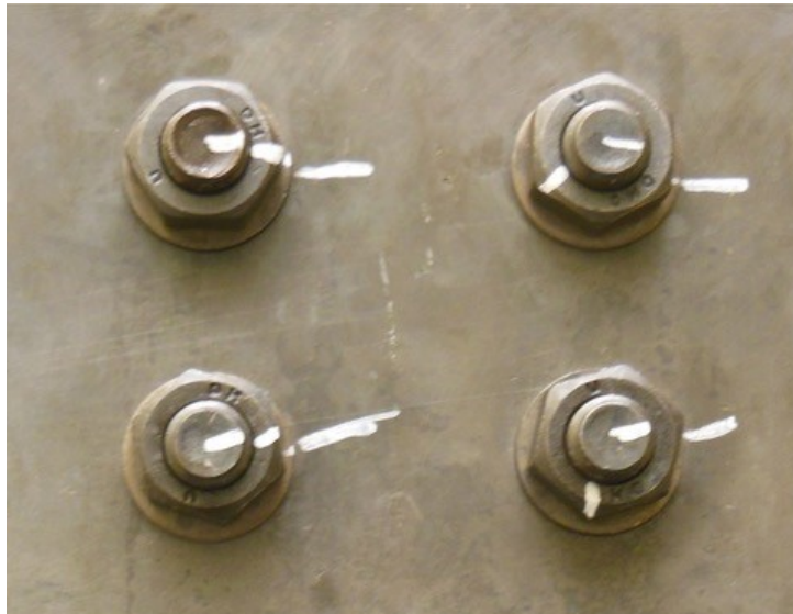
Figure 1: If the nuts are marked in this way with, for example, a white permanent marker, it will be clear if any have slipped. This is a quick and easy way to inspect your prototype before and after a test.
