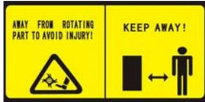
The rotating parts are sharp and running at high speed. Accidental contact can cause serious injury. Keep your hands and feet away from the parts while engine is running. Stop the engine and disengage the tines clutch before inspection or maintenance of the tines. Disconnect the spark plug cap to prevent any possibility of accidental starting, Wear heavy gloves to protect your hands from the tines When clearing the tines or then inspecting or replacing the tines.
