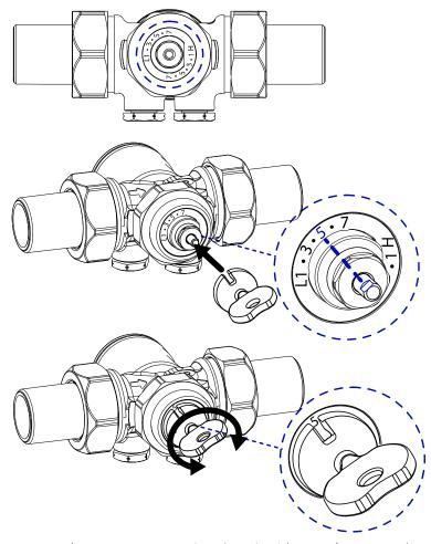
The BS9250015/20/25 valves are equipped with a double regulation scale of the flow rate:
