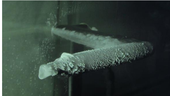
Figure 14. Iced-surfaced pitot tube [7]
