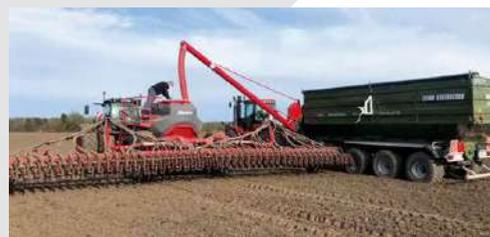
CHARGEMENT DES SEMOIRS PAR TUYAU PVC
