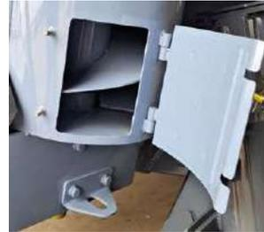
UNE TRAPPE POUR LE NETTOYAGE DE LA VIS SANS FIN VERTICALE
