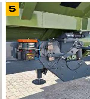
ORDINATEUR PROGRAMMABLE AVEC INTERVALLE PRÉCIS DE LUBRIFICATION DES ROUEMENTS
