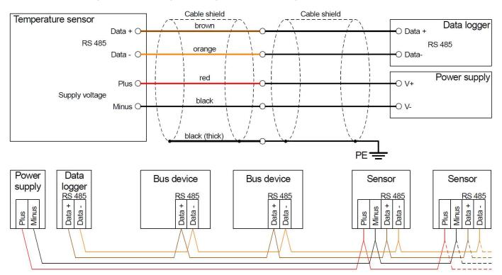
All MODBUS devices require the same bus parameter (baud rate, data format) but different addresses. Termination of RS485 bus usually is not needed.
