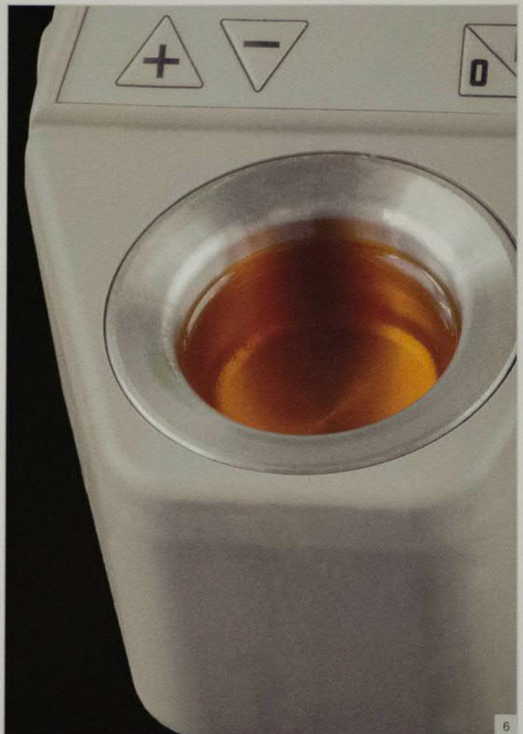
Fig 5-6 The electric dipping pot (Hotty, Renfert) with the dipping wax melted according to manufacturer recommendations.
