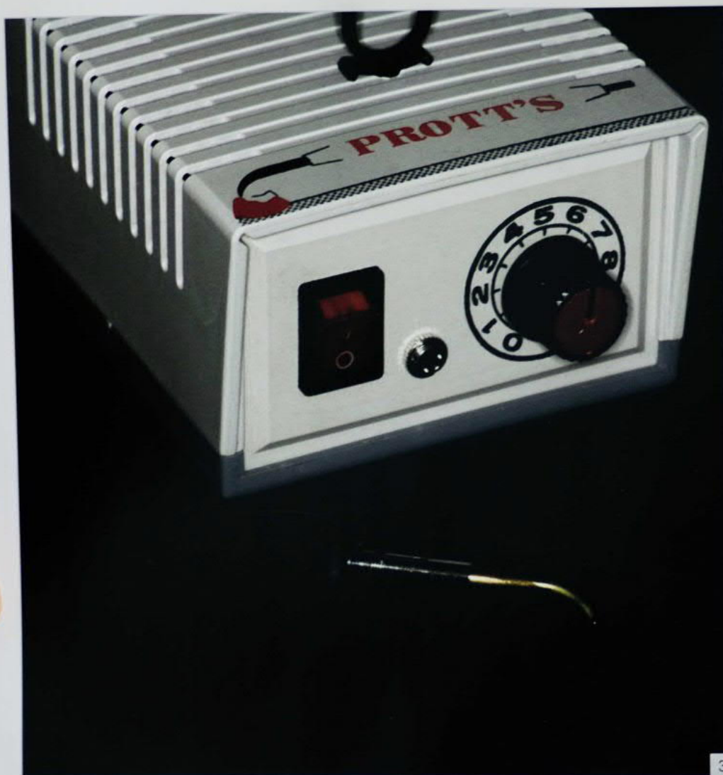
Fig 3-4 Molten wax for the sculpting process. The temperature can be set to provide the ideal viscosity. The wax must not be too fluid; otherwise, it will flow off the instrument. In that case, the temperature must be reduced.
