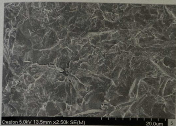
Fig 8-5 SEM image of a feldspathic ceramic (Creation). The crystalline portion is encased in a silica-rich matrix easily dissolved by hydrofluoric acid.
