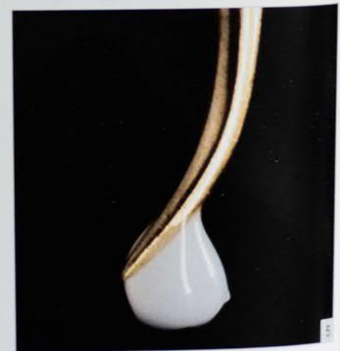
Fig 3-4 Molten wax for the sculpting process. The temperature can be set to provide the ideal viscosity. The wax must not be too fluid; otherwise, it will flow off the instrument. In that case, the temperature must be reduced.
