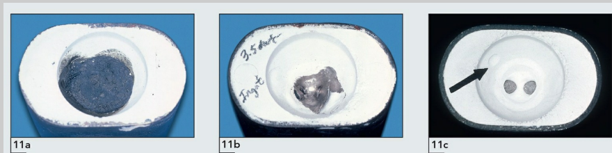
Fig 5-11 As one is able to better estimate the amount of alloy needed in the buttonless casting technique, the size of the cast button (a) will get smaller and smaller (b) until it is completely eliminated (c). Note the small concavity (arrow) formed in the investment by the wax orientation dot.
