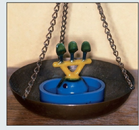
Fig 5-12b Wax buttons can be purchased to fill the opening in the top of the crucible former.
