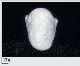
Fig 6-17a Although the manufacturer’s directions were followed, bubbling of the opaque porcelain occurred on this high-palladium–copper alloy.
