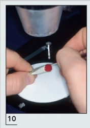
Fig 4-10 Use some form of magnification (such as a microscope, shown here) whenever possible to critically evaluate your work, whether you are assessing the intaglio surface of a wax pattern, marginating a wax pattern, or attaching sprue formers. Contemporary microscopes with flexible arms are available to facilitate the inspection of laboratory work.
