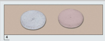
Fig 9-4 Polishing wheels (Cerami-Pro Universal Polishers, Brasseler). The porcelain prepolisher wheel (left) is gray and may look similar to a coarse stone wheel. It is designed for adjusting ceramic surfaces without leaving a rough surface. The final polisher wheel (right) is diamond impregnated and has a distinctive pink color. It is excellent for creating a smooth porcelain surface. Both wheels are available in round and knife-edge designs.
