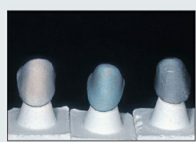
Fig 6-10 Three different base metal alloys: nickel-chromium-beryllium (left); nickel-chromium (beryllium-free) (center); and cobalt-chromium (right). Each casting produces a distinct oxidation when properly oxidized according to the manufacturers' recommended instructions.
