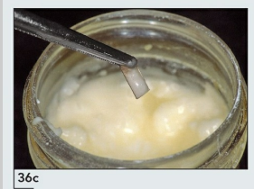
Fig 7-36c A fluoride-containing flux for presoldering (High Fusing Bon-dal Flux, Ivoclar Vivadent). A properly mixed flux should be moist and have a smooth, creamy consistency. Dip the cut solder strip into the presolder flux, and wipe off any excess so that only a light coating remains.
