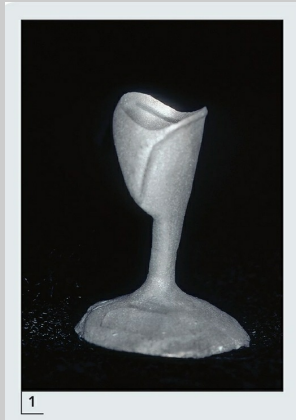
Fig 5-1 Casting produced using direct spruing. The straight sprue former can be modified with a ball reservoir, but the spruing method is still direct.
