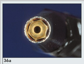
Fig 7-36a Single-orifice soldering tip on a Magic Wand torch (Ivoclar Vivadent).
