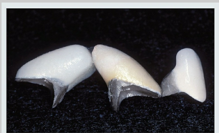
Fig 3-5a Three different brands of dental porcelain fired on copings made from the same palladium-silver alloy. The two nongreening porcelains (left and right) maintained their resistance to discoloration by silver after five body bakes, whereas the conventional porcelain (middle) took on a substantial yellow discoloration (particularly at the porcelain-metal junction) after just two firings.
