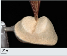
Fig 8-31e Sparingly apply the opaque modifier to the cervical region, and place a brown modifier in the interproximal region and on the occlusal surface (central groove area). Use the pointed brush to thin the occlusal line. Opaque modifiers on the cervical aspect of the substructure are visible from this occlusal view.
