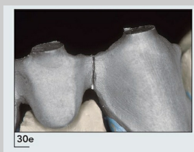
Fig 7-30e This gap is too small to allow for a sufficient amount of solder. It should be opened to approximately 0.3 mm for this high-palladium–silver–gold alloy.
