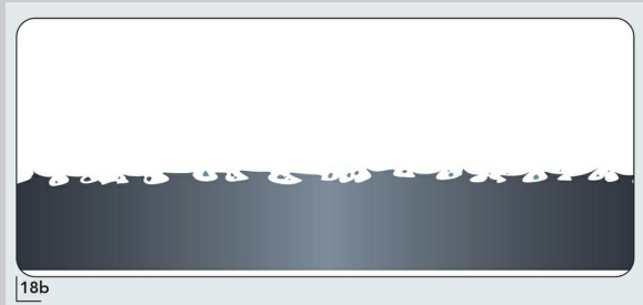
Fig 7-18b Some of the irregularities may retain debris that can later contaminate the porcelain.
