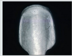
Fig 5-37 The same palladium-silver alloy shown in Fig 5-36b produced a smooth, complete replica casting based on a metal-ceramic substructure.
