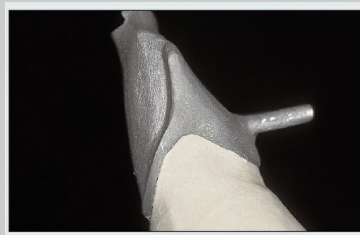
Fig 7-14 Lateral view of the casting seated completely.
