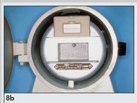
Fig 8-8b Interior of the front-loading porcelain furnace with a horizontal muffle. The operator works the vacuum manually as well as opens and closes the muffle door.
