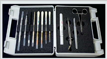
Fig 8-1a Porcelain kit (Renfert) containing the essential instruments for buildup procedures as well as for characterization (staining and glazing).
