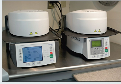
Fig 8-10a Programat P500 (left) and Programat P300 (right) (Ivoclar Vivadent) are examples of contemporary porcelain furnaces.
