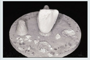
Fig 8-26 This wet porcelain buildup was not dried long enough or was suddenly exposed to high heat that produced steam and caused portions of the buildup to pop off the metal substructure.
