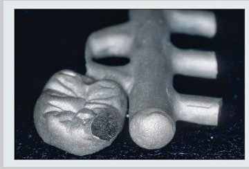
Fig 5-5a In this Type III gold casting, the large runner bar and the attached complete crowns (removed) were cast using a Tri-Wax sprue former (Ivoclar Vivadent). A runner bar of this size (4 gauge) is able to support large metal-ceramic pontics and retainers better than a smaller-diameter (6 gauge) runner bar. Note that the wax pattern was located off the runner bar by approximately 5 mm.
