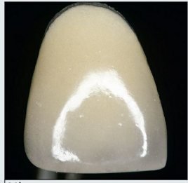
Fig 9-21b An overfired crown possesses an extremely reflective, glossy surface devoid of surface characterization and shows signs of rounding of previously sharp corners.
