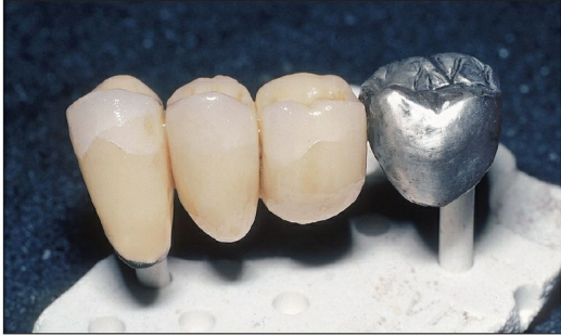
Fig 4-1 Crack formation in the porcelain veneer of all three units is evidence of stress, which was attributed to poor substructure design—specifically, too much freestanding porcelain.
