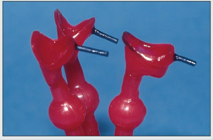
Fig 5-28 Before securing the patterns to the runner bar, it is recommended that you add 18-gauge wax to the lingual surfaces. This step creates handles in the cast framework, thereby protecting the delicate cast metal margins.
