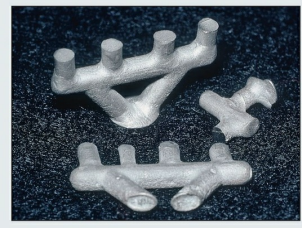
Fig 5-4b The cast indirect spruing network can be sectioned and reused more readily than can buttons of spent metal.
