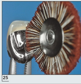
Fig 9-25 With a second, soft-bristle brush, pick up a small quantity of rouge compound. Lightly polish the metal with rouge compound until the surface takes on a high luster (compare to Fig 9-23e). The labial metal collar can be mechanically polished quite adequately with fine green polishing wheels or other fine abrasives.
