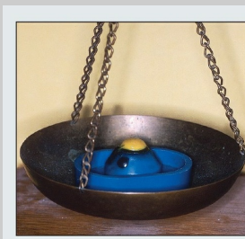
Fig 5-12a The opening in the crucible former is filled with wax and the orientation dot is placed. The crucible former is put on a scale and weighed. The weight of the crucible former is permanently
