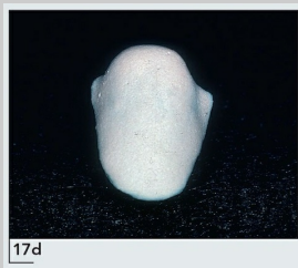
Fig 6-17d Merely refinishing this casting removed the surface and subsurface contamination and resulted in an appropriate porcelain-metal bond.
