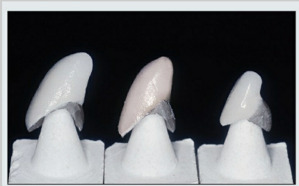
Fig 3-5a Three different brands of dental porcelain fired on copings made from the same palladium-silver alloy. The two nongreening porcelains (left and right) maintained their resistance to discoloration by silver after five body bakes, whereas the conventional porcelain (middle) took on a substantial yellow discoloration (particularly at the porcelain-metal junction) after just two firings.
