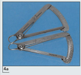
Fig 7-4a The measuring caliper for metal (Pfungst) (top) looks similar to the measuring caliper for wax (Pfungst) (bottom).
