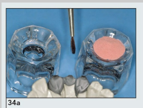
Fig 7-34a To join the metal components together, use an acrylic resin with low polymerization shrinkage, such as Pattern Resin LS (GC). Dispense a small quantity of powder and liquid in separate dampen dishes, and select a small, clean brush.
