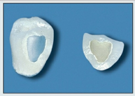
Fig 6-11 Porcelain-metal bond failures can occur through the oxide layer itself if that layer is too thick or poorly adherent. Note how the ideal straw-like color of the oxide layer remains bonded to the porcelain and cleanly separates from the metal surface.
