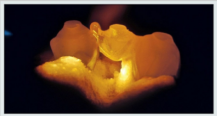
Fig 7-36g As heating continues, focus on the connector area, and watch as the head of the tadpole disappears as the solder slumps and flows into the prepared connector area.
