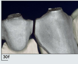
Fig 7-30f This solder gap is larger than the desired 0.3-mm gap distance.
