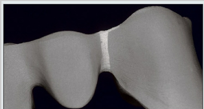
Fig 7-40 Close-up view of the solder joint after oxidation. The yellow hue of the presolder is now readily apparent, and the solder joint is dense and free of contamination and porosity.
