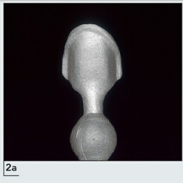
Fig 7-2a The completed casting should be dense and free of defects. Note the smooth transition from the sprue to the restoration, which is a direct result of the care taken during spruing.
