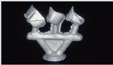
Fig 5-30 This casting has fins caused by excess wax pattern cleaner or improper heating of the mold.
