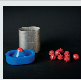
Fig 5-12c A prefabricated wax sprue former, with attached wax patterns, is placed in the crucible former, and the entire assembly is weighed.
