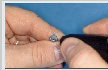
Fig 7-13 Grind the marked area on the inside of the casting using a small carbide bur in an electric handpiece and light, intermittent pressure.
