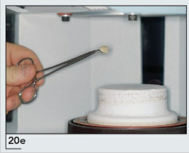
Fig 9-20e Carefully and slowly dry the restoration in the porcelain furnace muffle entrance.
