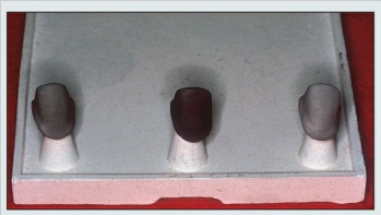
Fig 6-9 These three oxidized copings were made with noble alloys, yet their color and character (eg, texture, thickness) appear to be markedly different. The Olympia casting (Jelenko) (left) is medium gray and has a moderate level of oxidation. The high-palladium–copper alloy Naturelle (Pentron) (center) has the darkest color (dark brown to black) and the highest level of oxidation. The Ivoclar
