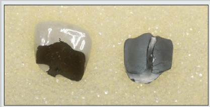
Fig 6-13a Note how the heavy greenish oxides are bonded to the porcelain (left), yet a substantial amount of oxidation remains on the metal substructure (right) of this cobalt-chromium casting.
