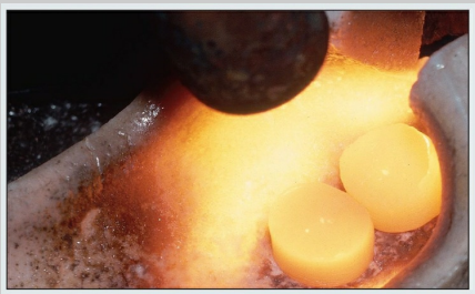
Fig 5-33b Through mutual contact, the ingots can heat uniformly.
