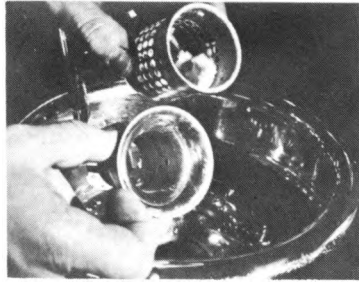
Figure 429.—Cleaning out trap.
