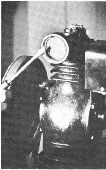
Figure 478. —Removing the retaining ring for filter.
