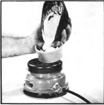
Figure 373. —Plaster or stone mix vibrated into box.
