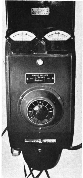
Figure 168.—Panel of General Electric wall-mounted X-ray unit.
