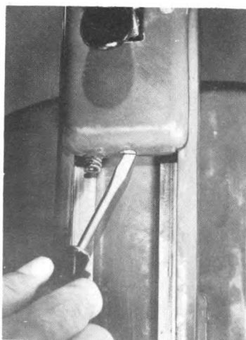
Figure 464.—Tightening headrest slide setscrew.
