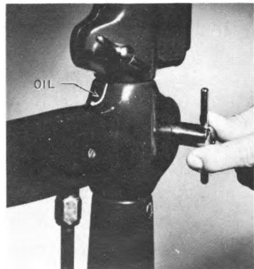
Figure 423.—Loosening the adjusting nut.
