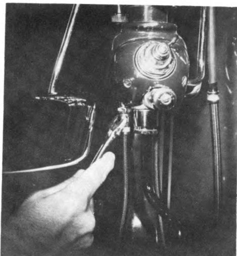
Figure 431.—Loosening ejector tubing.
