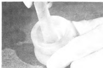
Figure 309. —Use of the glass mortar and pestle.
