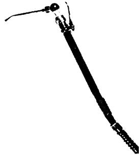
Figure 441.—Spring hose protector disengaged.
