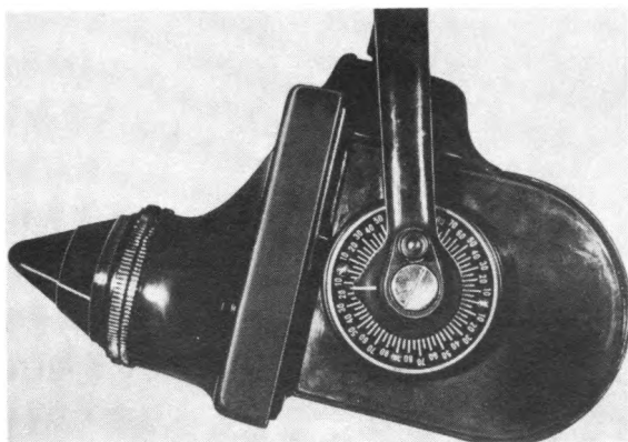
Figure 182.—X-ray unit head with a minus 15 degree setting.
