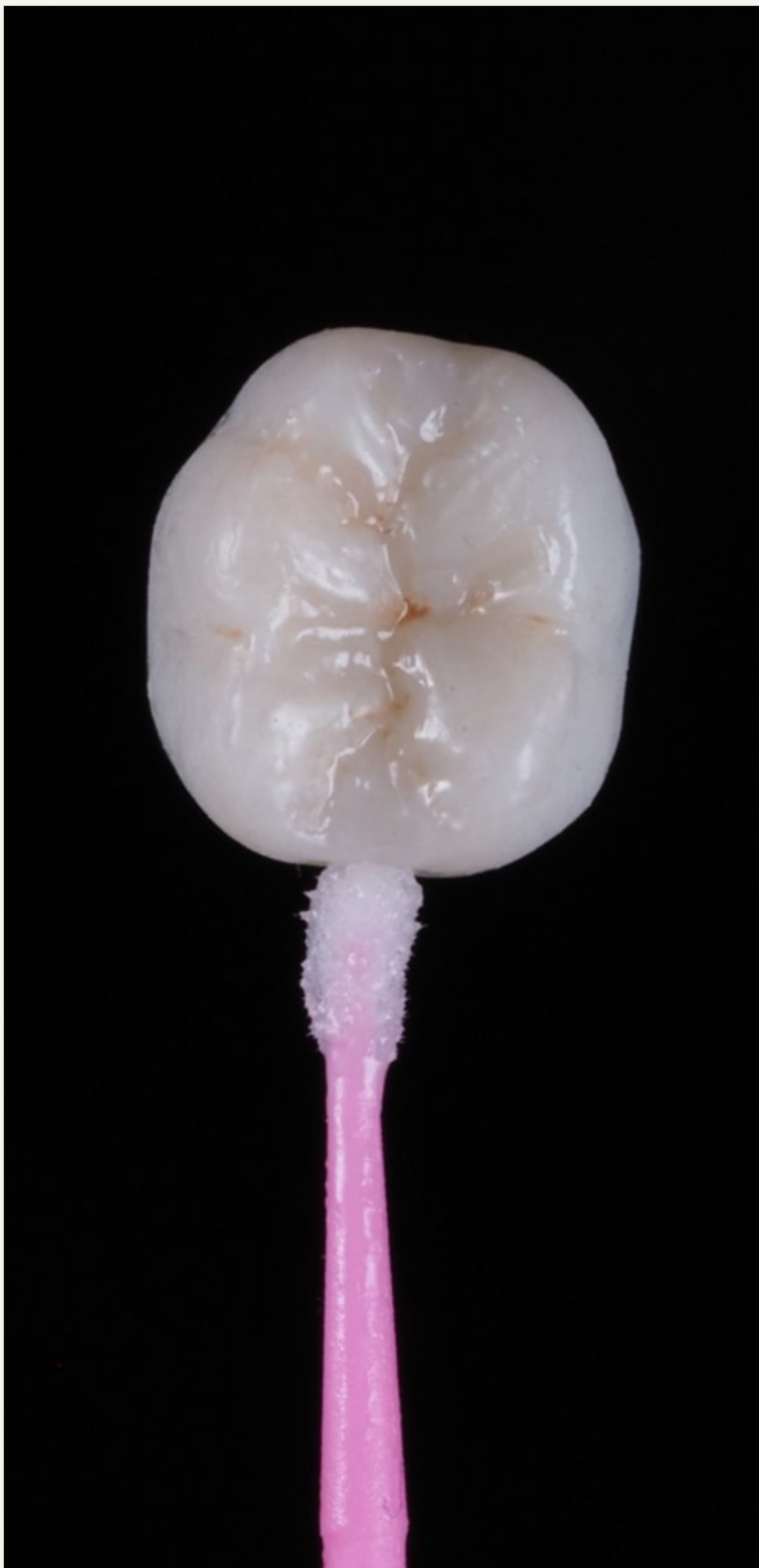
3D printed Crown fabricated on the Ackuretta SOL using Rodin Sculpture resin
