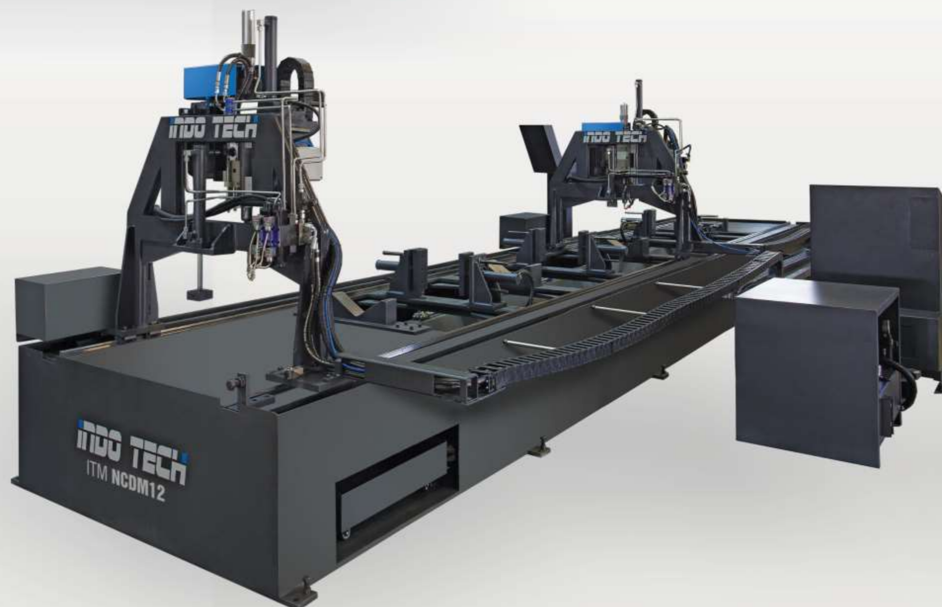
Multiple Fixed Hydraulic Clamping vices with V-block resting.
