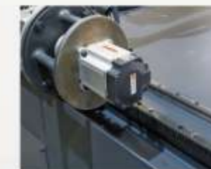
Cutting Arm Feed thru Hi-End Servo System & Feed Back thru Rack & Pinion.
