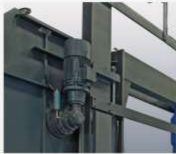
High efficiency power transmission to Saw through PLANETARY GEAR BOX
