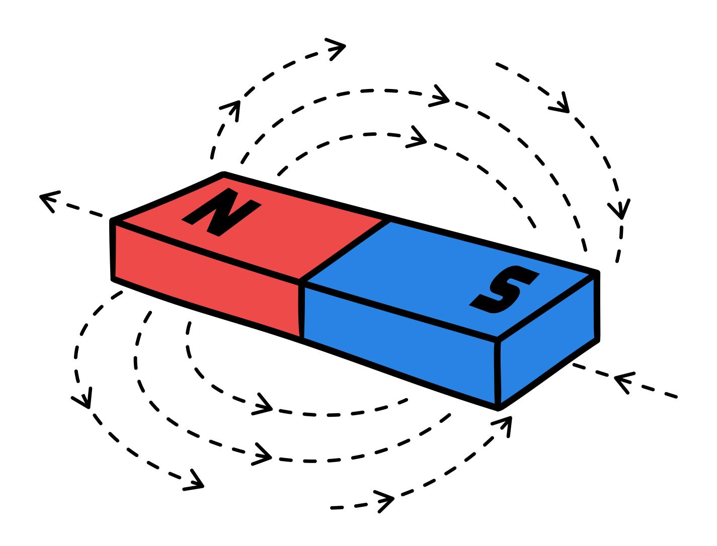
Magnetic force is the push or pull made by a magnet. It can attract or repel objects like iron or another magnet. This happens because of the magnetic field around it.
