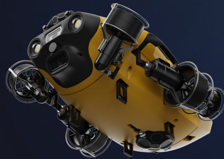
Main ROV Unit ×1 (incl. Forward Q-DVL/Range Laser & Downward Q-DVL)
