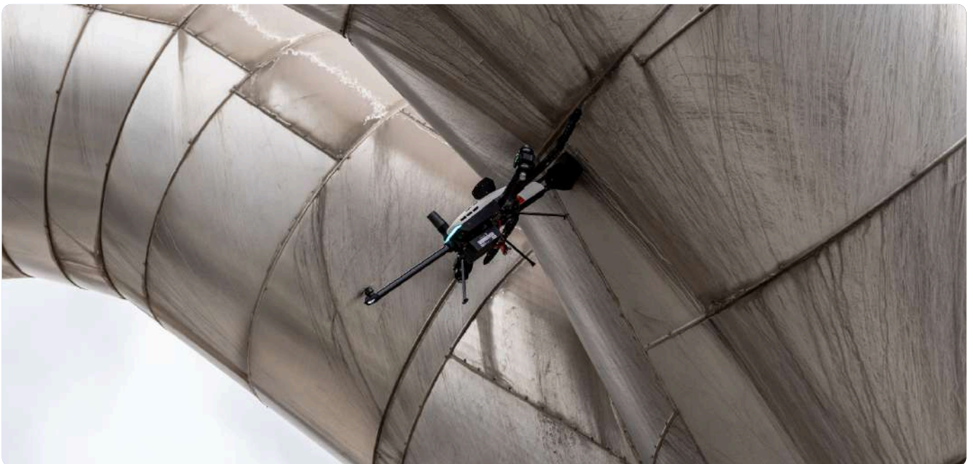
The Voliro T PEC sensor takes measurements through insulation and aluminum jackets, eliminating the need to proactively remove insulation
