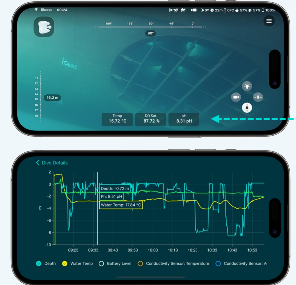
Aqua TROLL 500 fitted on the Blueye X3. Data parameters integrated in the Blueye App.
