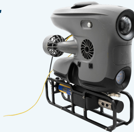
Aqua TROLL 500 fitted on the Blueye X3. Data parameters integrated in the Blueye App.
