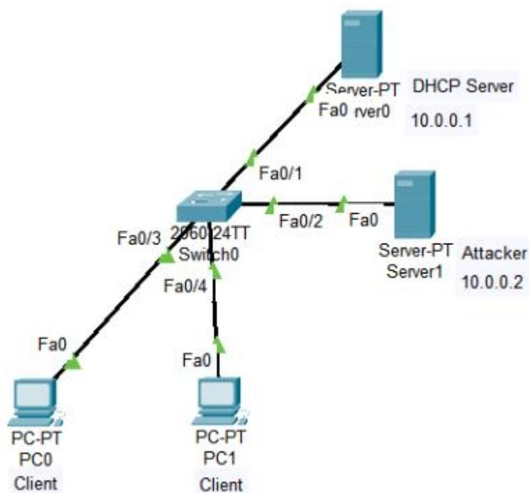
**Task 1:** Connect the above network, assign IP addresses to the DHCP server and the attacker as depicted in the figure. Then enable dhcp snooping in the switch, and make sure that port1 is dhcp snooping trusted port.
