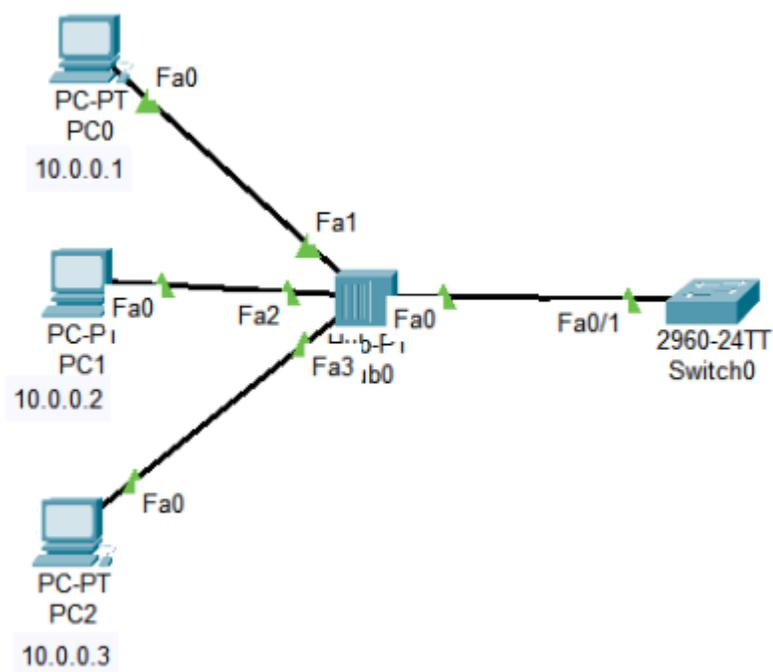
**Task 1:** Connect the network as shown in the diagram, and assign IP addresses to the PCs as depicted. Then Configure Port 1 in the switch with port security enabled, and try to make a ping from two different PCs and check the port is moved to down state due the security violation.
