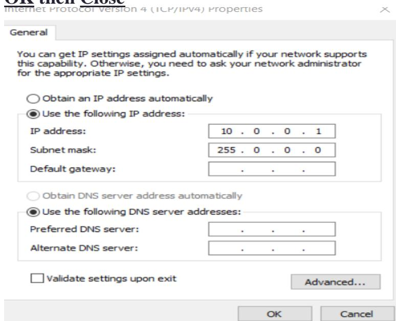
**Task 7: Repeat the above process for PC\_B, by assigning it IP 10.0.0.2 255.0.0.0**
