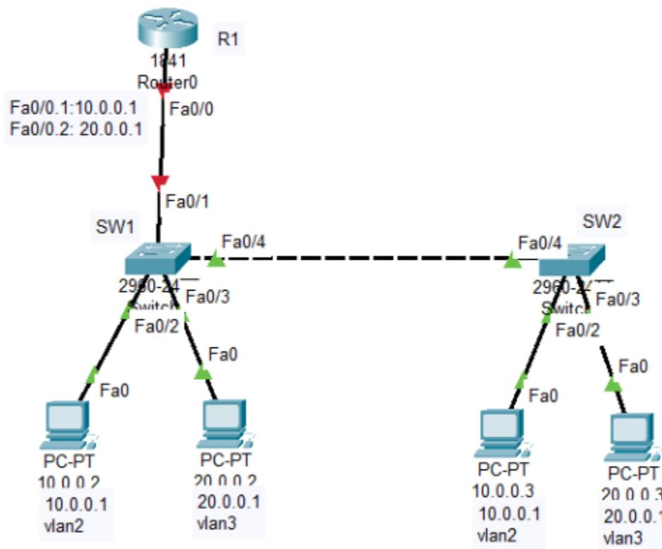
**Task 1:** Connect the above network, create vlans on the switches and assign the relevant ports, configure the trunk link between the switches and between SW1 and the router. Then configure the router as router on stick as depicted in the diagram. Use the following show commands for troubleshooting
