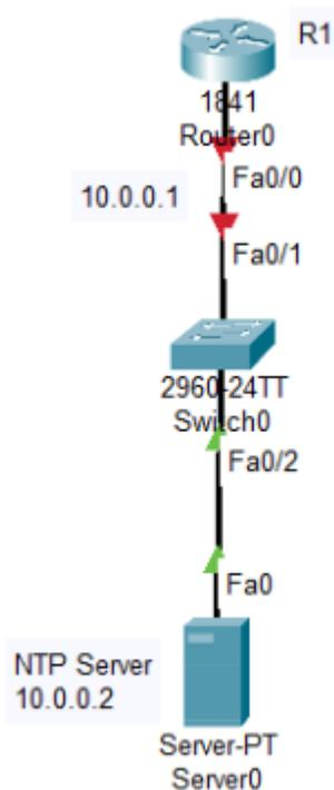
**Task 1:** Connect the network as shown in the above topology, assign IP addresses. Configure the Server as NTP Server, and the router as NTP Client, and verify the ntp configuration
