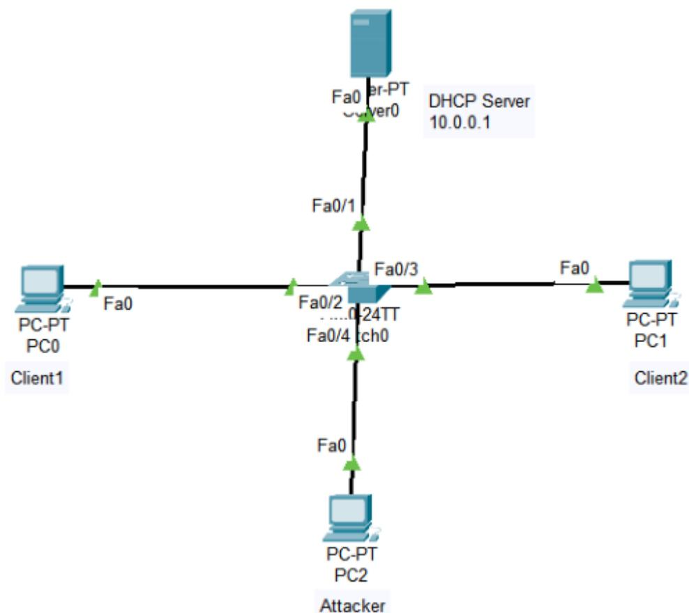
**Task 1:** Connect the network as shown in the diagram, enable the DHCP server to dynamically assign ip addresses to the client starting 10.0.0.10. Before connecting the attacker to the network, assign it ip address similar to client1 then connect the attacker to the network. Make a ping from the attacker to Client2, and you can notice the ping is working
