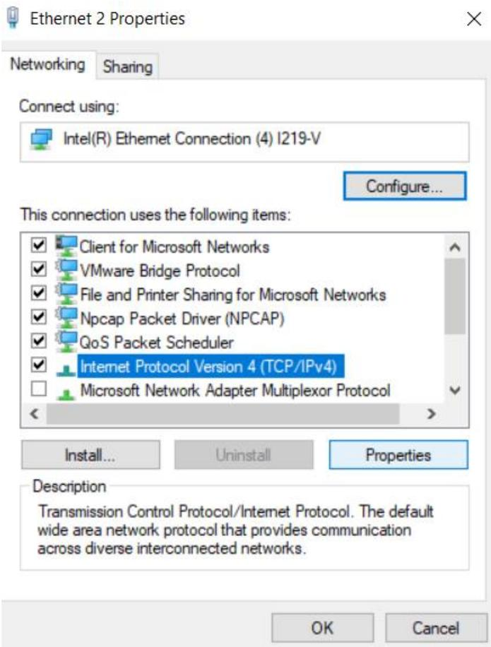
**Task 6: Then Assign IP addresses as shown below with the subnet mask and choose OK then Close**
