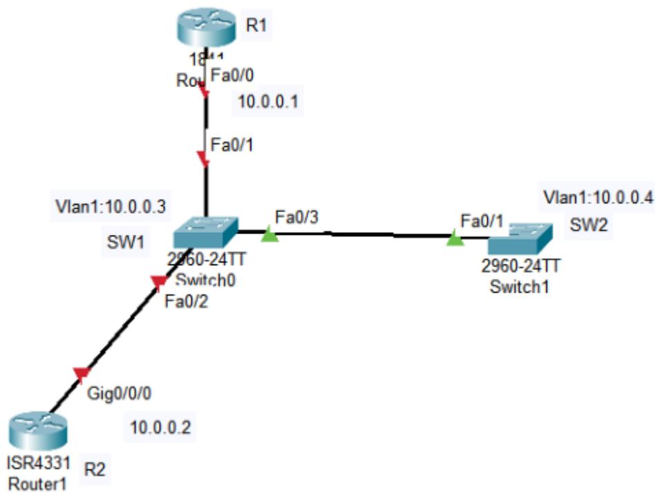
**Task 1:** Connect the above network, and assign IP addresses as shown in the figure, and verify the cdp neighbor status
