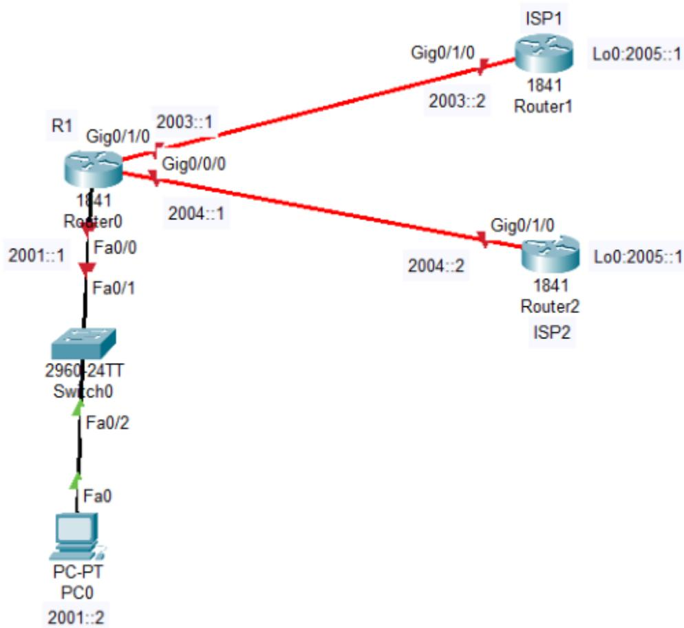
**Task 1:** Connect the above network and assign IP addresses as depicted. Configure ISP1 & ISP2 for reverse static routes pointing to 2001::/64 network. Then configure R1 with floating default routes by making ISP1 is the preferred route.
