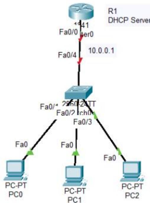
**Task 1:** Configure R1 as DHCP Server, and ensure that all PCs connected to the switch are getting IP address dynamically
