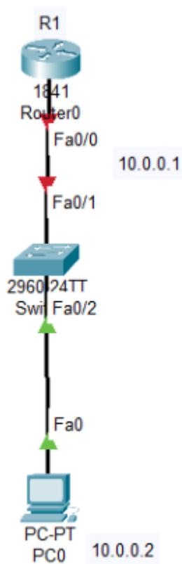
**Task 1:** Connect the above network, and configure R1 to be ssh enabled with local username and password as authentication method.
