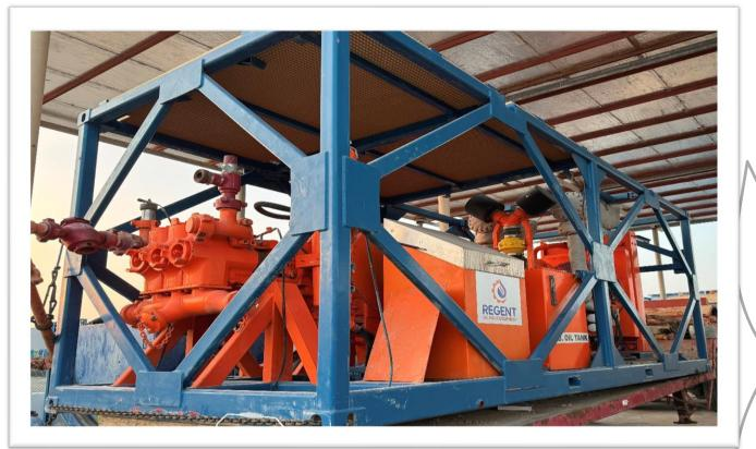
New custom made heavy-duty crash frame with forklift pocket, certified pad eye and lifting slings, control panel mounted on platform for controlling, bet better unit supervision and maintenance purposes, epoxy coated
