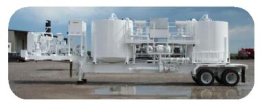
Batch Mixer Mounting Trailer is mainly used for slurry mixing of onshore and desert oilfield cementing jobs, especially those with critical requirements of the slurry. This unit mainly consists of the trailer, engine, pump drive, centrifugal pumps, batch mixing tanks
