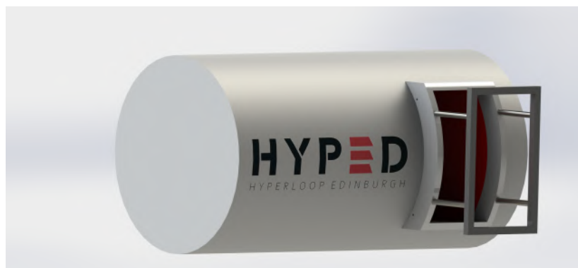
Figure 35: CAD render of bridge doors airlock capture system attached to a pod
