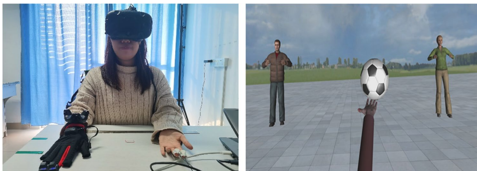
Fig. 1 Experimental setup. Left panel: Participants wore a head-mounted display on their head and an orientation tracker and data glove on their right hand. Skin-conductance response electrodes were attached to the index and middle fingers of the left hand; the keyboard
