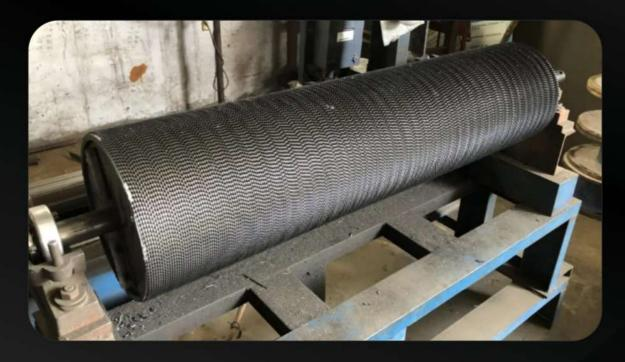
Carding wire being mounted on carding roller/drum of carding machine before carding process
