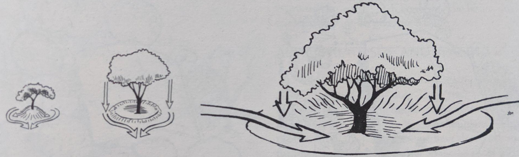
Fig. 5.3. From left to right, a tree planted atop a mound from which water and soil drain away; within a circular berm which diverts area runoff and any leaf drop falling outside the berm away from the tree; and within an infiltration basin toward which the surrounding area is sloped so all direct rainfall, surrounding runoff, and leaf drop is harvested. These trees could've all been the same size at planting, and planted at the same time, though their current size reflects how the vegetation will respond to the degree to which different landforms drain or harvest resources.
