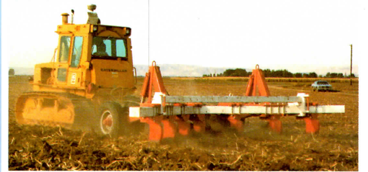
Crawler tractor shown pulling 42" shanks for additional trash clearance.
