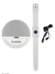
Remote assistance device for calling recorded numbers via mobile network. The hands-free call is sent by pressing the "Alarm" button or using the push button on the bracelet/pendant accessory supplied or another device connected to the interface 03895. The device can also receive incoming calls with automatic answering
